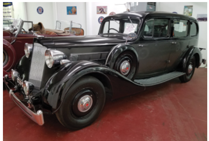
An "English" version of a 1936 Packard Super-8 Touring Limousine complete with right-hand drive and English style headlamps.
