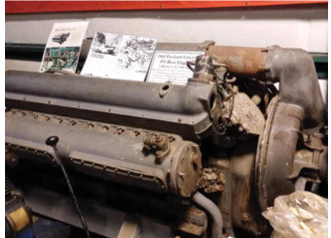
The 2,490 cid, 1,500 bhp V12 Packard Liberty engine. Three of these were used to power a PT boat during WWII.
