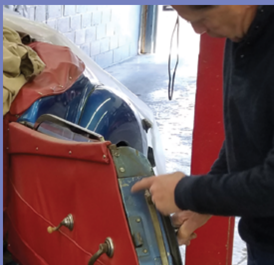
The very first Darrin prototype – 1938. Ralph shows the crudeness of the work. The seat is not attached to the floor and the seatback is held up by a leather covered brick.
