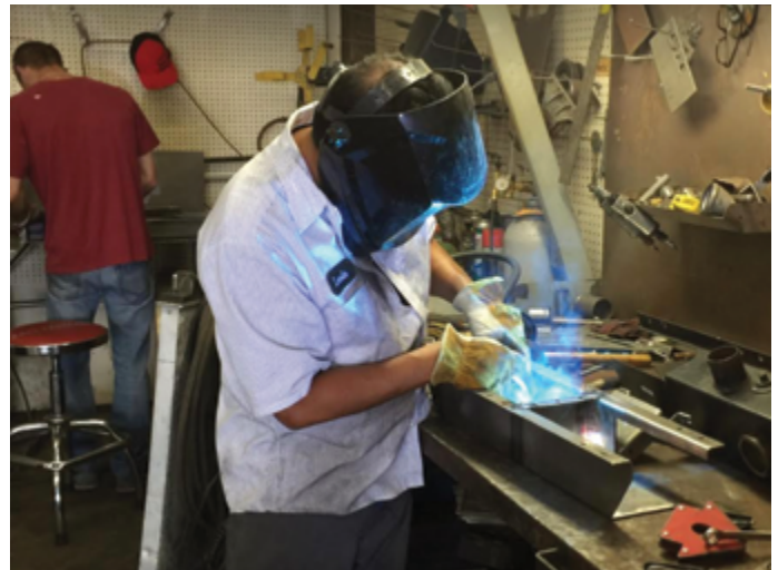
Will Garrett fabricating an Ice Box Performance radiator that fits perfectly into the stock radiator’s location.
