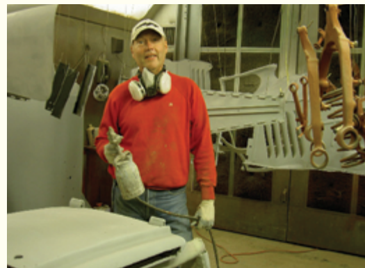
Priming parts in the paint booth at Becker's DIY Restoration
