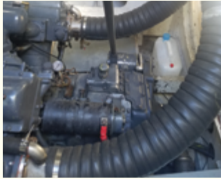
A 6" diam. exhaust pipe for each bank of cylinders
